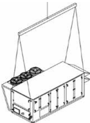
Lifting Details for XRV 20, 40, 85, Applies to units with or without side air return
