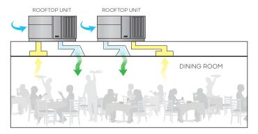
A traditional design utilizes HVAC Rooftop Units (RTU). A dining space requires a certain amount of ventilation to temper the space, as well as a certain amount of outside air based on size and occupancy. Due to the limitations on outside air capacity on RTUs, multiple units are typically required. This often results in oversupplying, requiring more diffusers and ductwork.
