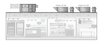
You can simplify the space by replacing multiple RTUs with fewer DOAS units, simplifying controls and reducing installation costs.
