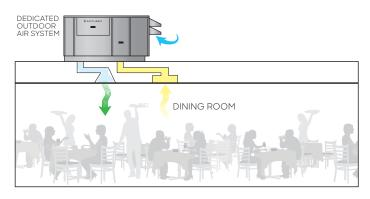
Since a DOAS unit is designed for high percentages of outside air, you can typically reduce the number of installed units as well as design the unit to supply the exact amount of air necessary to meet code and desired space conditions. This reduces the number of units, ductwork, and diffusers required.
