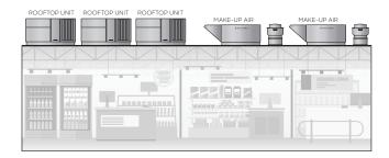
With many hoods in operation exhausting large amounts of air, many RTUs would be necessary to meet code requirements for outside air and keep the space comfortable and safe. More RTUs mean more roof penetrations, higher installation costs, and more complicated control scenarios.
