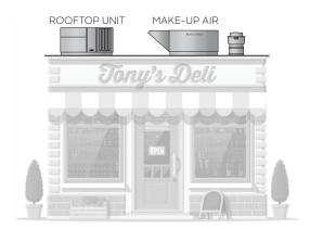
With the limited tempering capacity of a rooftop unit, the effect of minimally tempered, high-percentage outdoor air from the MUA may dominate the space. Without adequate temperature and humidity control, a small space gets uncomfortable fast and display cases quickly fog up.
