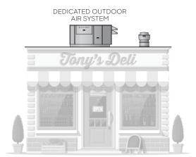
By replacing the multiple units with a single DOAS unit, you can ensure precise temperature control throughout the space and still make up the high amount of outside air required from the kitchen hood.
