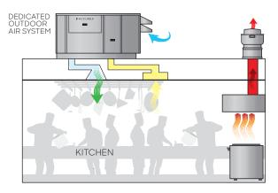
A DOAS unit can combine the functions of a make-up air unit and RTU in the kitchen, potentially allowing you to replace the need for both with a single unit. A DOAS unit also removes moisture before entering the kitchen, versus trying to control it after.
