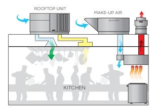
A traditional design utilizes both Make-up Air (MUA) and HVAC Rooftop Units (RTU). MUA is typically used to 'make up' around 80% of air exhausted through the hood. The RTU over the kitchen is used to make up the rest and condition the kitchen space. With RTUs there are limitations on the capacity of outside air they can handle.
