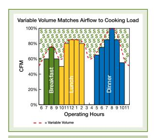
A variable volume system will track the cooking load (dashed red line) and vary the exhaust and supply ventilation. The area above the red line represents energy savings.
