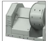
**Drive Assembly** – Machined, cast iron pulleys are factory set to required RPM and are adjustable for final system balancing for applications with 10 hp or less motors. Sized for a minimum of 150% of driven horsepower.
