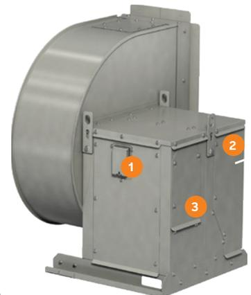
**UL/cUL 762** – The UL/cUL 762 option includes a weatherhood, threaded drain connection and access door. Indoor mounting requires the fan to have welded scroll construction.
