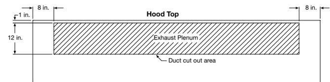
2. The exhaust duct connection is to be a continuous liquid-tight weld. Utilizing the 1" (rectangular collars) or 1/2" (round collars) flange, weld with a non-ferrous filler wire, such as silicon bronze or stainless steel filler wire. Protect all stainless steel areas from weld splatter.
