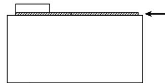
Three inches (7.62 cm) uninsulated airspace installed on top of hood (optional) meets NFPA 96 requirements for clearance to limited combustible surfaces.
