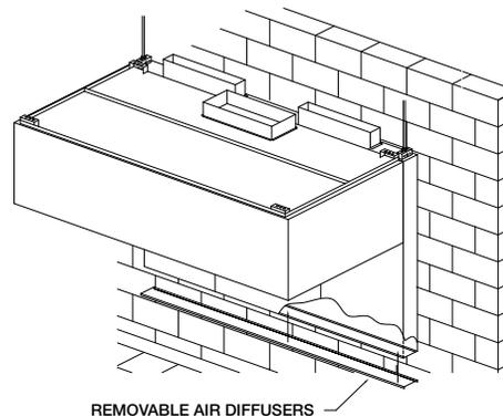
1. To clean the air diffusers, unfasten the screws. Remove the air diffusers from the back supply unit and wash in the sink or dishwasher.
