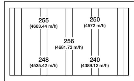
$$\text{Average Velocity} = \frac{\text{Sum of Velocity Readings}}{\text{Number of Readings}}$$
