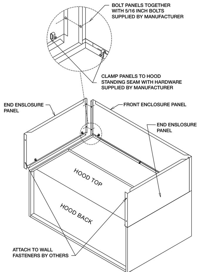
TACK WELD OR USE SELF-TAPPING SCREWS (PROVIDED BY OTHERS) TO SECURE FRONT ENCLOSURE PANEL AND PART OF THE SIDE ENCLOSURES TO TOP OF ASP
