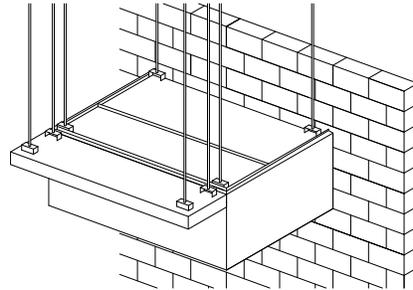
1. Insert 1/2 in. (12.7 mm) diameter threaded rod (by others) into hanger brackets on the external supply plenum top. Raise and hang the external supply plenum from adequate roof or ceiling supports.
