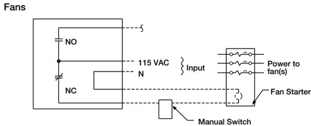
If prohibited by local codes, do not shut down exhaust fans with this method of wiring.
