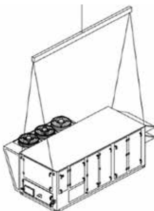
Lifting Details for XR 10-45, Applies to units with or without side air return Lift from the top of the unit 4 lifting points.
