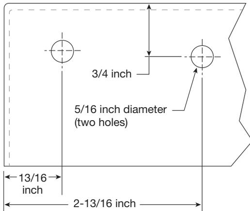
2. Attach “L” shaped hinge bracket to curb cap with two 1/4 inch-20 x 3/4 inch bolts per bracket. Leave finger tight until all pieces are installed. Refer to Figure 3.
