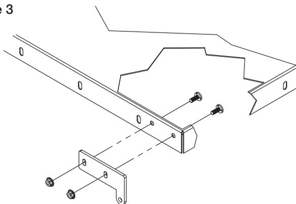
3. Center curb cap on curb. Ensure there is equal space between curb and curb cap on all sides.
