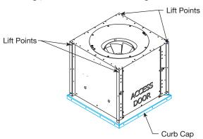
• **NOTE:** Image shown is for supply configurations, with the inlet of the fan up. Exhaust configurations would have the outlet of the fan up.
