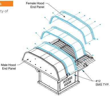
Align inner hood panels by overlapping the female rib of the panel on top of the male rib of the previously installed panel. Be careful not to damage the panels. Use a rubber mallet to help interlock the hood panels together.
