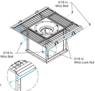
Align the hole in the L-bracket of the hinge assembly with the hole at the end of the hood support rail and the hood support angle.
