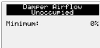
Occupied and unoccupied damper control have minimum and maximum set points for the specific mode of operation. Unoccupied OA Damper control typically will only show the minimum set point. The maximum will also appear if the OA Damper is controlling to building pressure.
