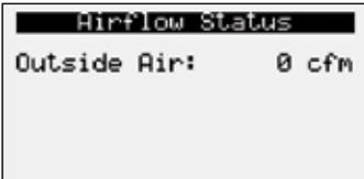
The GreenTrol® airflow monitoring station measures airflow using advanced thermal dispersion technology. An integral LCD display provides a local indication of airflow measurement and device configuration. The airflow monitor also features Modbus communication allowing the microprocessor to monitor the airflow as well. The GreenTrol also accepts up to two airflow probes for averaging.
