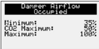
**Minimum Position** – When in the occupied mode, the active setpoint will be equal to a local minimum OA setpoint, which may be constant or reset by fan speed if equipped with a modulating supply fan.
