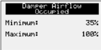
This screen only appears if equipped with a modulating OA and recirculating damper. The screen displays the min and max positions for the outside air damper. These setpoints reflect the percentage of the outside air damper being opened.
