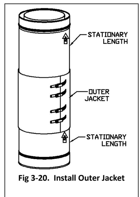
Fig 3-20. Install Outer Jacket
