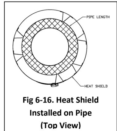
Fig 6-16. Heat Shield Installed on Pipe (Top View)
