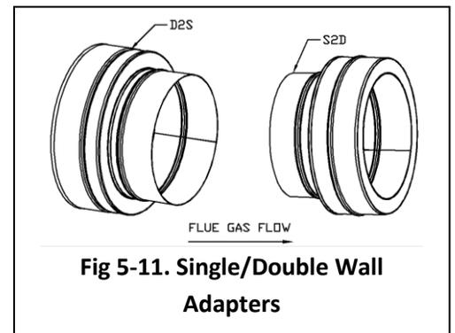
**Fig 5-11. Single/Double Wall Adapters**
