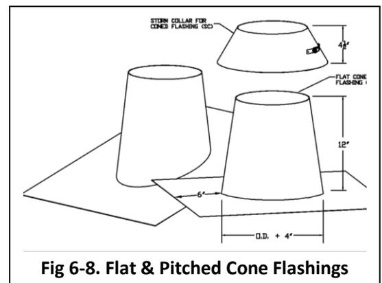
**Fig 6-8. Flat & Pitched Cone Flashings**
