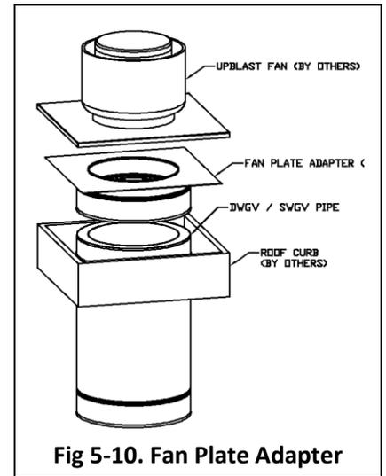
**Fig 5-10. Fan Plate Adapter**
