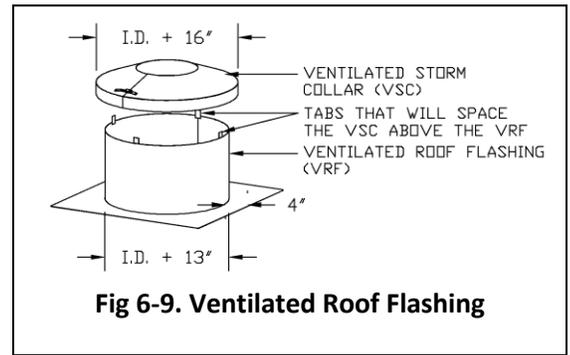
**Fig 6-9. Ventilated Roof Flashing**
