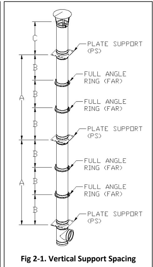
Fig 2-1. Vertical Support Spacing
