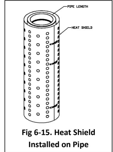
Fig 6-15. Heat Shield Installed on Pipe
