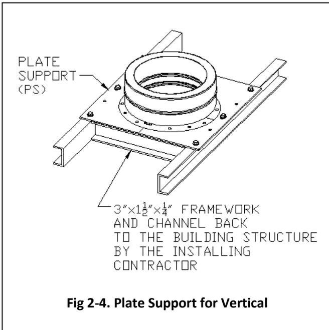
**Fig 2-4. Plate Support for Vertical**
