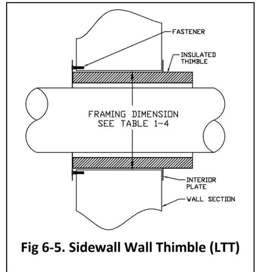
**Fig 6-5. Sidewall Wall Thimble (LTT)**
