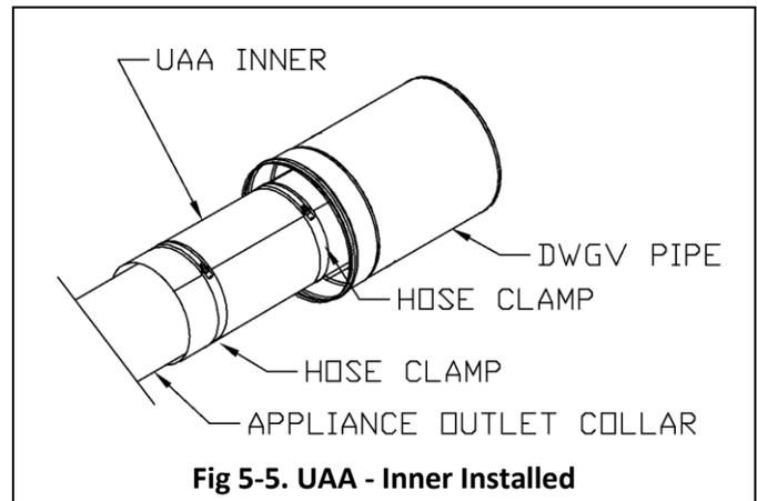
**Fig 5-5. UAA - Inner Installed**
