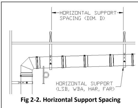
Fig 2-2. Horizontal Support Spacing
