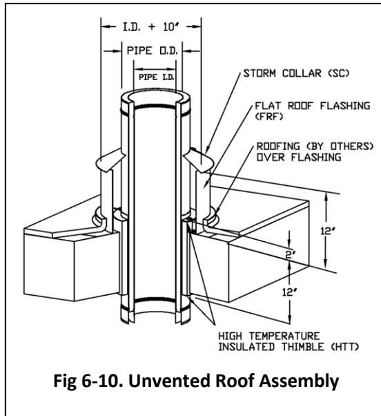
**Fig 6-10. Unvented Roof Assembly**
