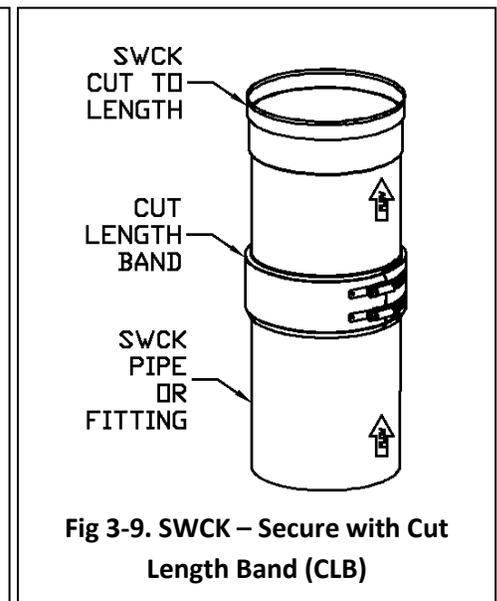
Fig 3-9. SWCK – Secure with Cut Length Band (CLB)
