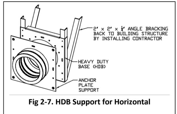
**Fig 2-7. HDB Support for Horizontal**
