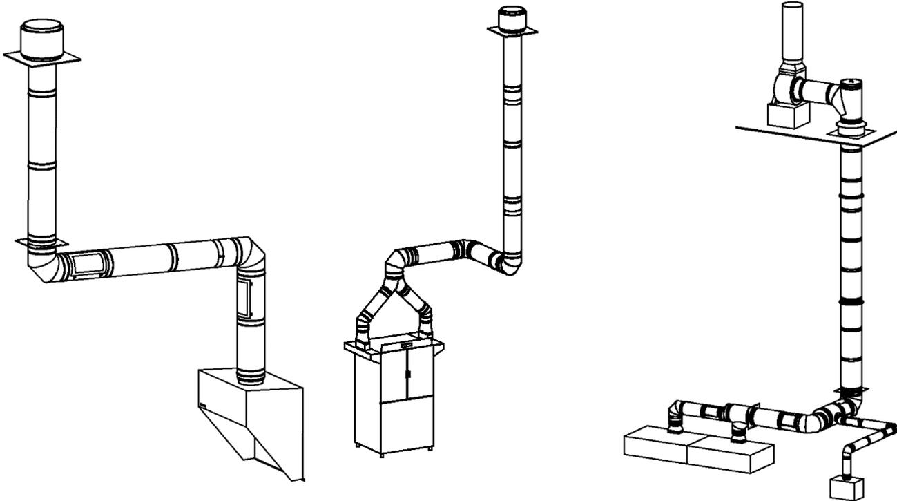
**A MAJOR CAUSE OF VENT RELATED FIRES IS FAILURE TO MAINTAIN REQUIRED CLEARANCES (AIR SPACES) TO COMBUSTIBLE MATERIALS. IT IS OF THE UTMOST IMPORTANCE THAT JEREMIAS CK SYSTEMS BE INSTALLED ONLY IN ACCORDANCE WITH THESE INSTRUCTIONS.**
