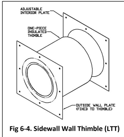
**Fig 6-4. Sidewall Wall Thimble (LTT)**
