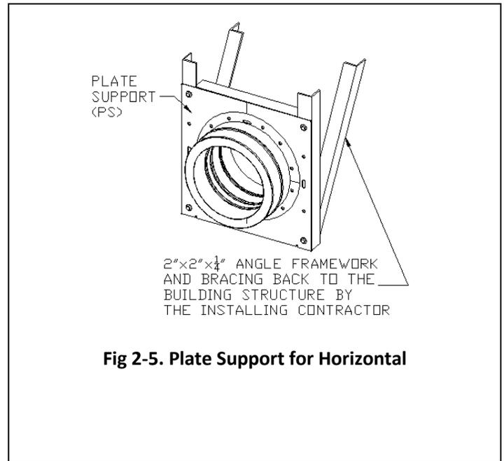
**Fig 2-5. Plate Support for Horizontal**
