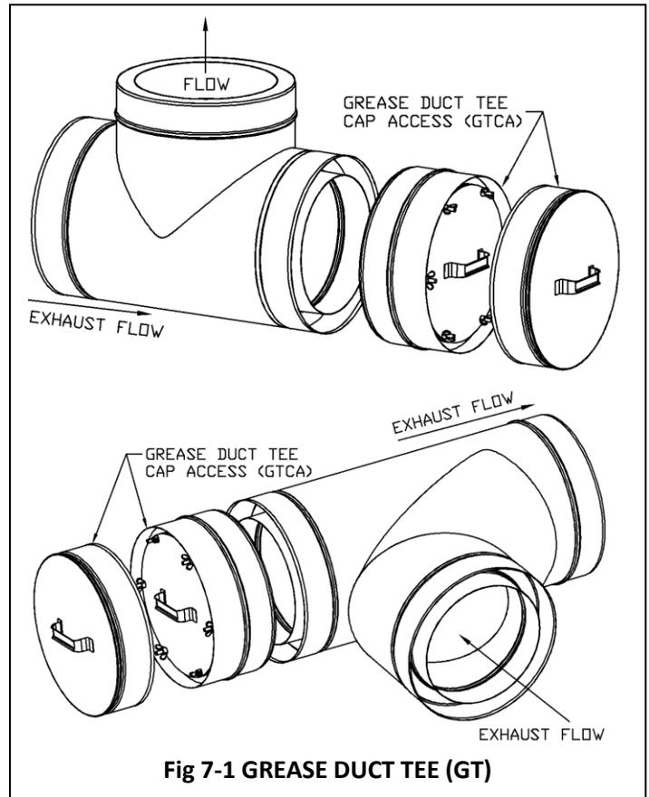
Fig 7-1 GREASE DUCT TEE (GT)
