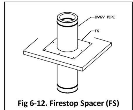
**Fig 6-12. Firestop Spacer (FS)**
