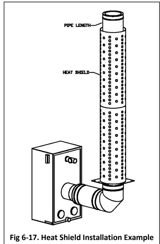
Fig 6-17. Heat Shield Installation Example
