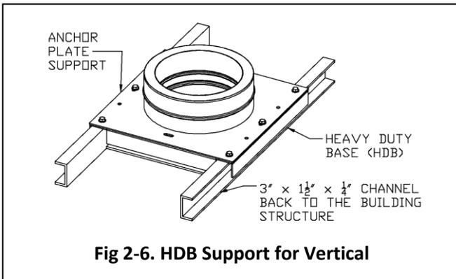
**Fig 2-6. HDB Support for Vertical**
