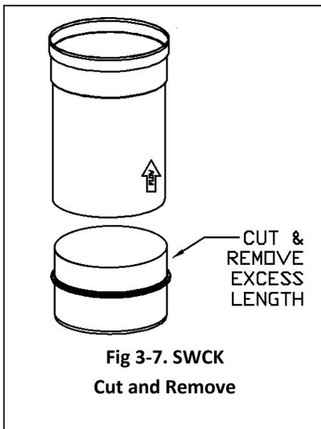
Fig 3-7. SWCK Cut and Remove
